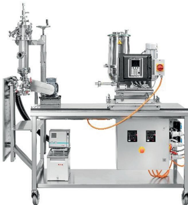
Figure 2: D-Lab, laboratory thin film dryer used for drying CTA and PTA in our lab in Switzerland
